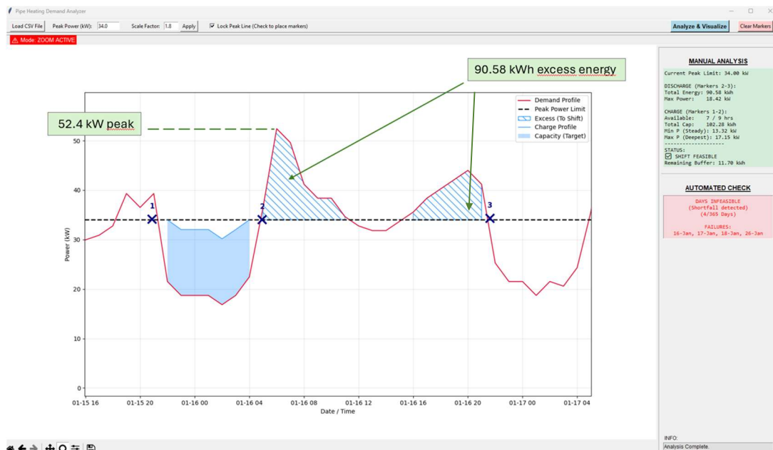
Figure 25: Determination of the heat that needs to be stored decentrally with the purpose to eliminate the analysed peak in the network using the PeakAnalyser Tool. Example from 15 January to 17 January for customer #10 of the Landiswil DHN with highlighted information that is needed for the further design steps in THENA.
