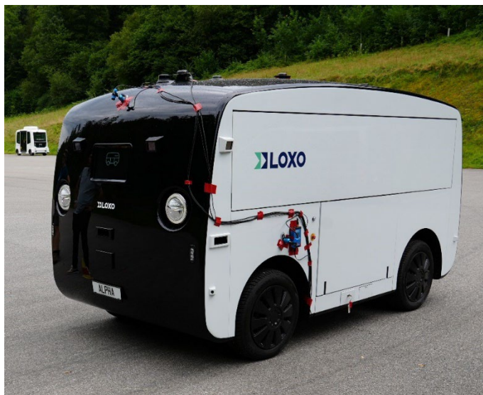
Figure 78: Antenna and camera positioning on LOXO Alpha
