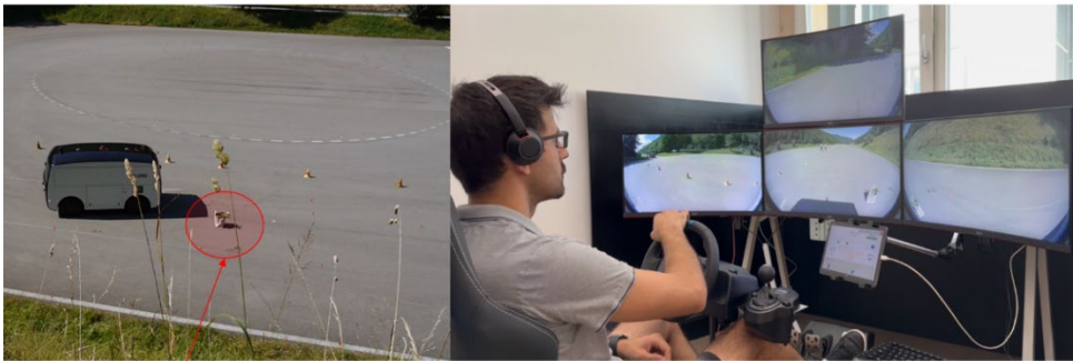
Fig-S 7: Scenario 8 - False positive obstacle detection - solution bypassing ROL2
