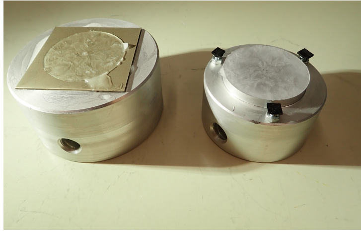
Figure 4.6: Ice adhesion test with force perpendicular to the sample surface: cohesive ruptures in the ice lead showing remaining ice on both sides: coating (left) and upper sample holder (right).
