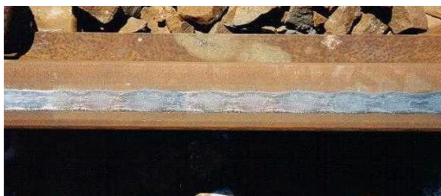
Abbildung 2-2 Short pitch corrugations on the running surface (aus [8])
