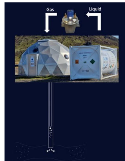
Figure 4. Schematic representation of the injection process at the Hellisheiði site.
