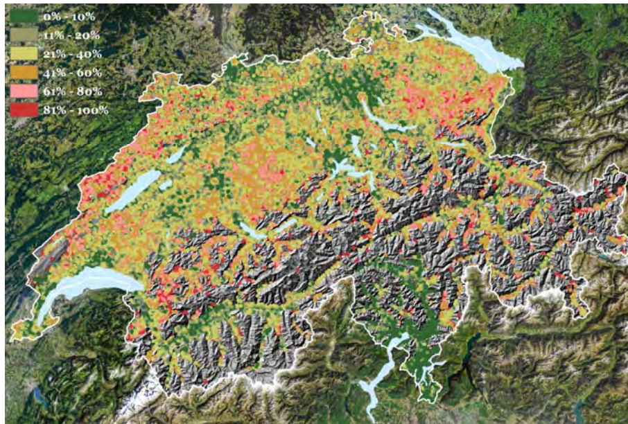
Figure 1: Spatial probability of housing stocks (built before 1919), cell size (X, Y): 25m, 25m, r=1000m
