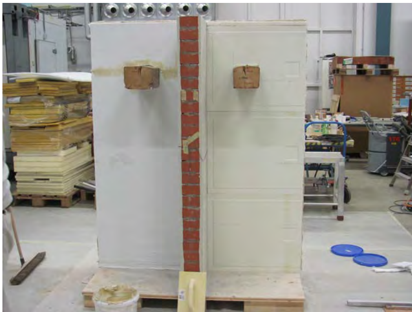
Figure 23: Test wall for accelerated weathering tests at Empa. Two different aerogel insulation layers are applied. Wooden beam heads in the test wall represent the most critical detail for internal insulation.
