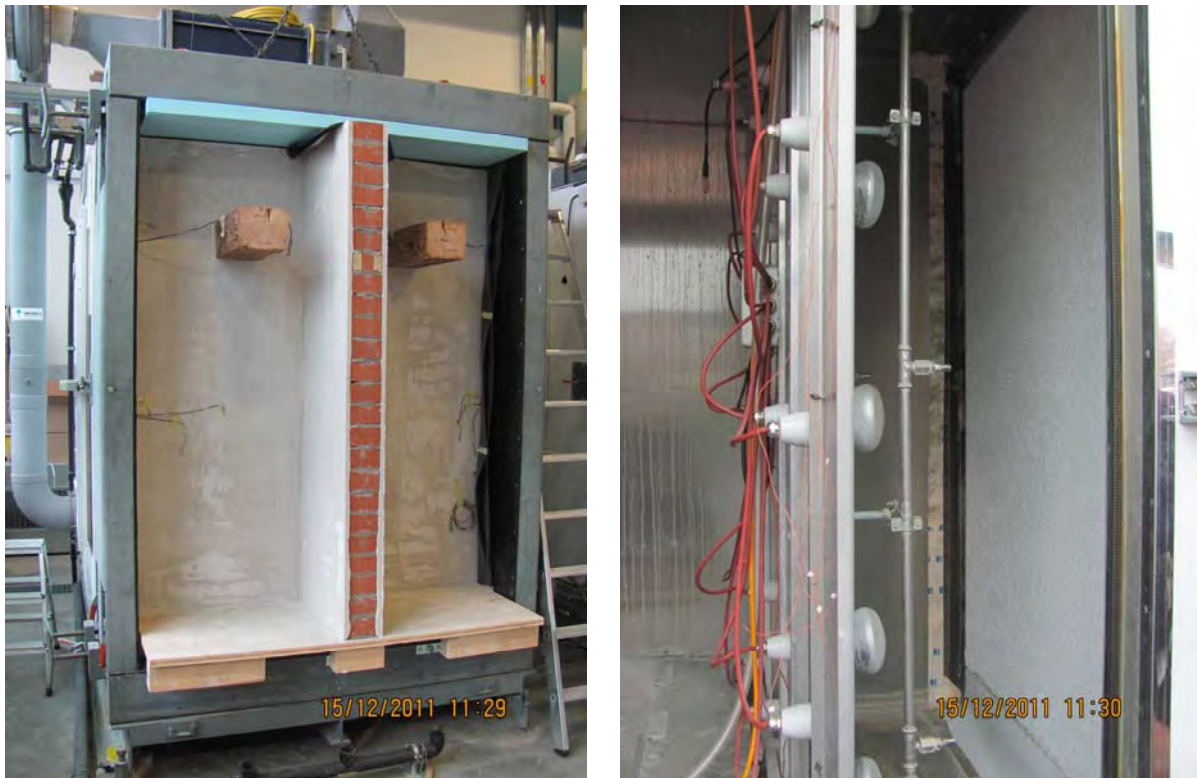
Figure 24: The test walls have been exposed to rain, sun and frost cycles in Empa’s weathering chambers and temperature (right, inside view of testing chamber) and relative humidity profiles were measured across the wall.
