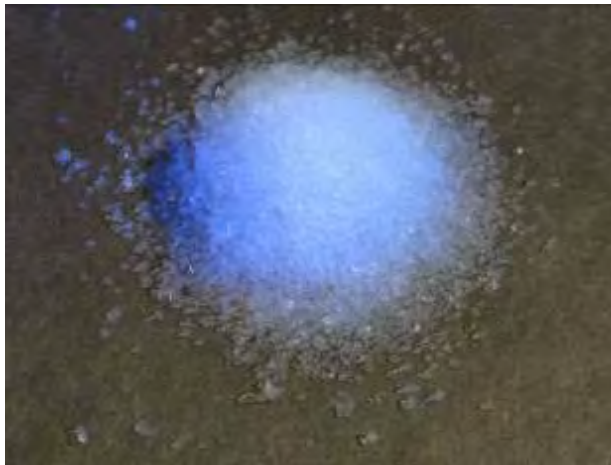
Figure 12: About 85% nanoporous aerogel granulate is used as additive for the light weight plaster
