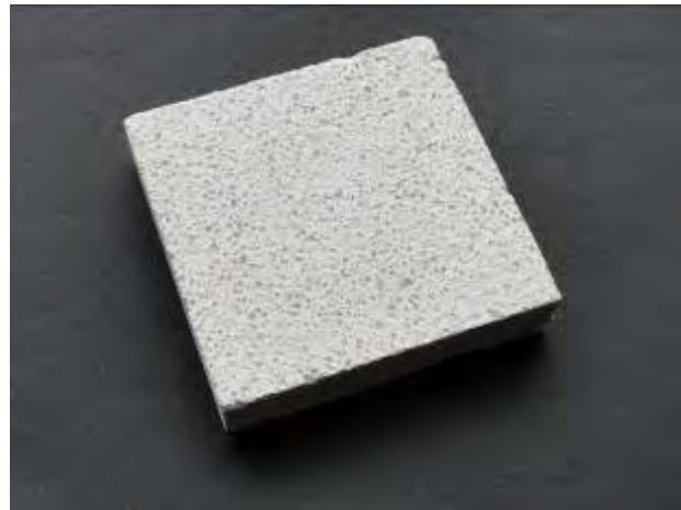
Figure 13: Sample of the highly insulating rendering. The pores are filled with transparent nanoporous Aerogel
