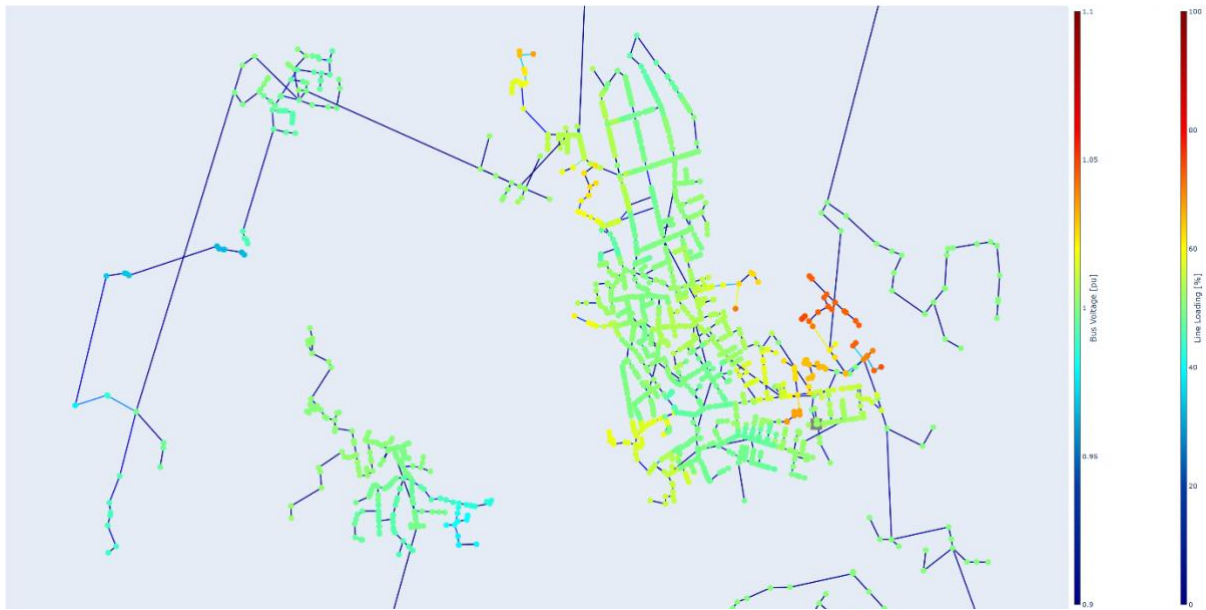
Figure 14: Graphic representation of the distribution grid state with color gradients for bus voltages and line loading showing the result of a 100% flexible EV fleet reacting to the Vario 6 tariff at 12 PM
