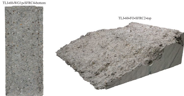
Fig. 6.5 - Vertical transverse cut through half specimen TLJ-60-WG1p-SFRC4 after testing and failure plane of half specimen TLJ-60-FO-SFRC2.
