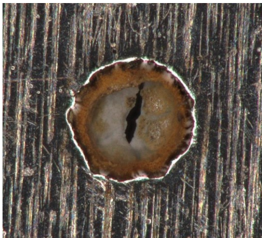
Figure 12: Photo of the HMX-1 laser cut distributing hole, clogged with debris.
