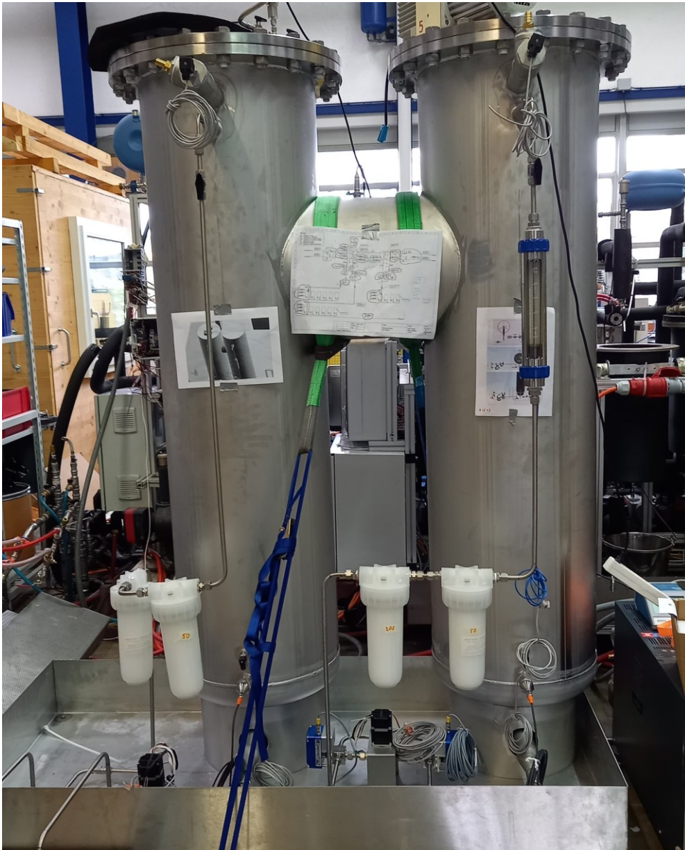
Figure 7: Photograph of HMX-1 installed for laboratory testing at HSLU. The left vessel contains the absorber/desorber section, while the right vessel contains the evaporator/condenser section.
