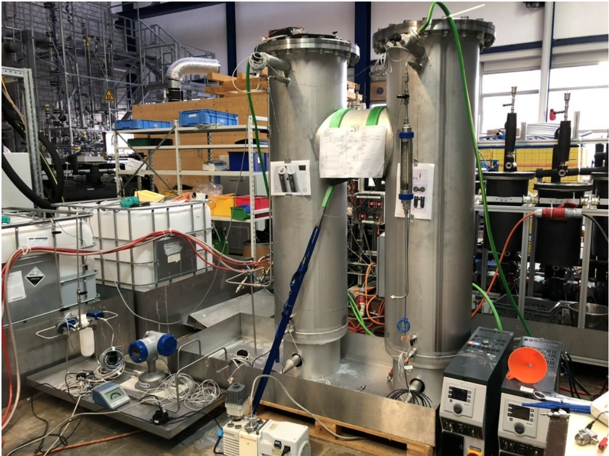
Figure 14: Photograph of HMX-1 at HSLU. The heat and mass exchanger, comprising two cylindrical stainless-steel vessels with flange lids, is prominently visible near the centre-right. On the left side, the sorbent tanks are displayed, with the front tank containing the charged sorbent.
