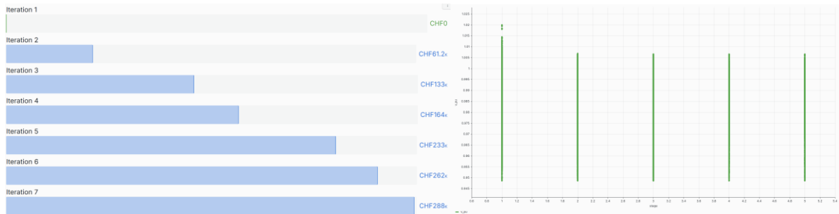
Figure 55: The convergence plot together with stage wise comparison of voltage variation of Feeder Aumont.
