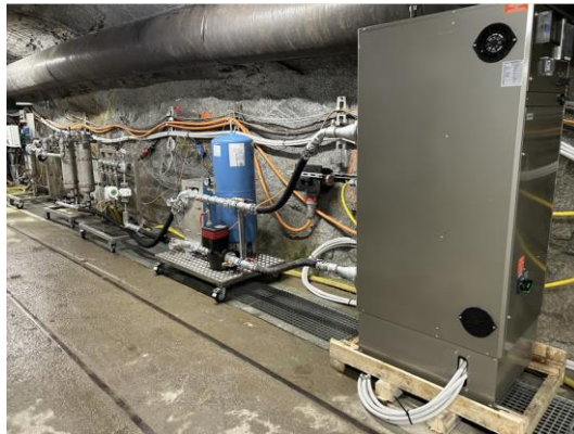
Figure 7: Left: Jaspi flow-through heater with separate heat exchanger circuit. Right: array of six high-pressure injection pumps with a combined capacity of up to 270 L/min.
