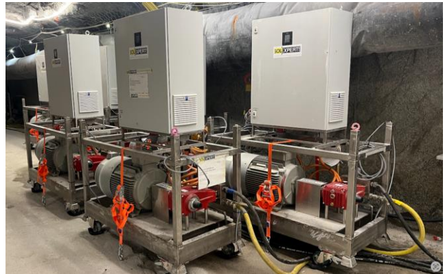
Figure 7: Left: Jaspi flow-through heater with separate heat exchanger circuit. Right: array of six high-pressure injection pumps with a combined capacity of up to 270 L/min.
