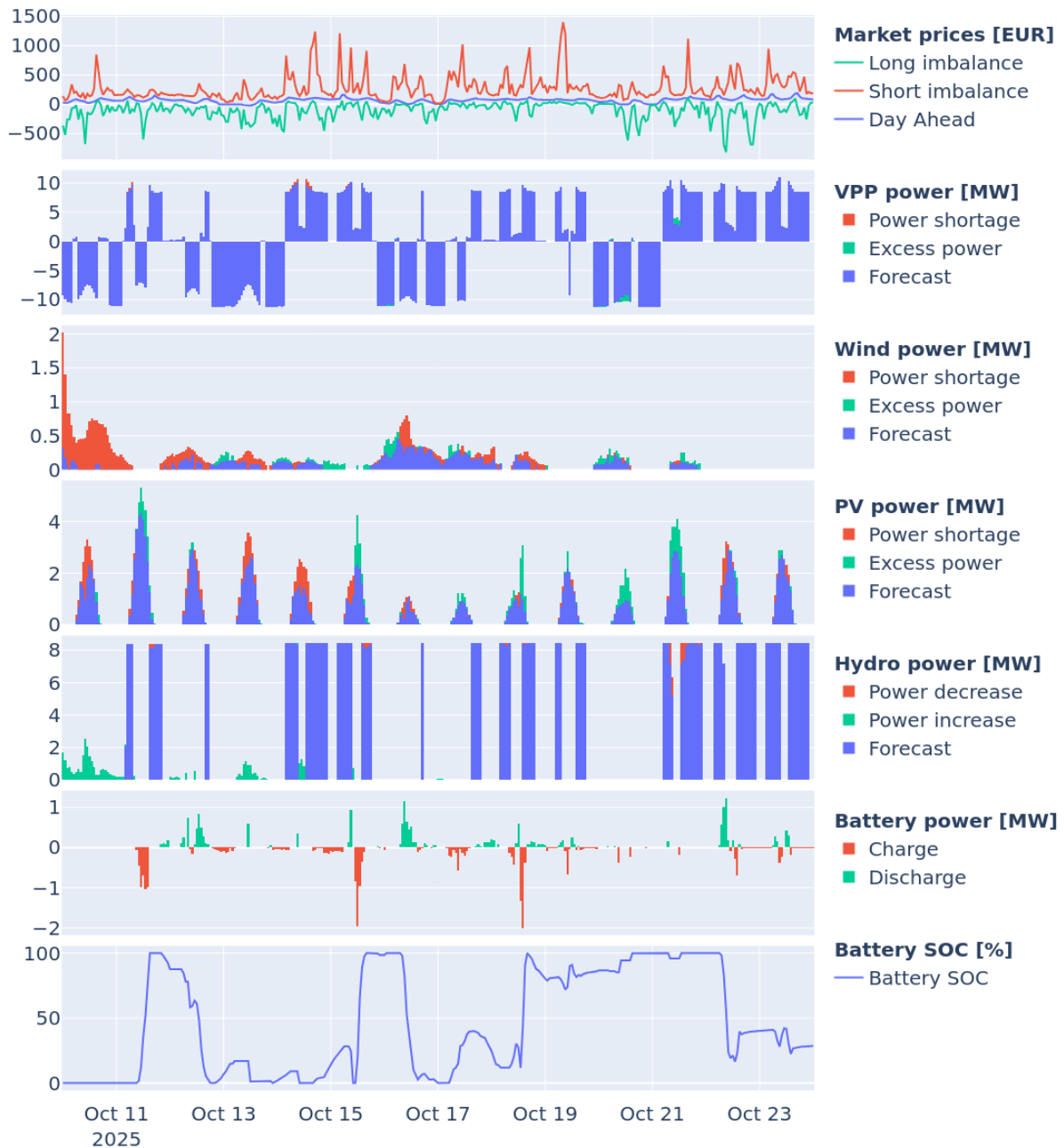
Figure 126: Two-week zoom on third-stage optimization results, highlighting forecast errors and their reduction using a continuous turbine and a 2 MW / 4 MWh battery
