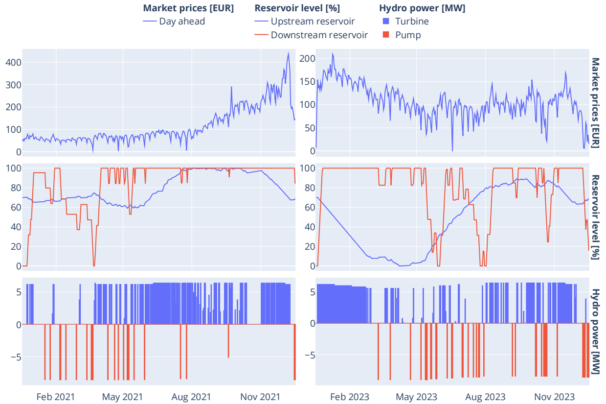
Figure 117: First-stage optimization results for the years 2021 (left) and 2023 (right) with a discrete turbine and a pump
