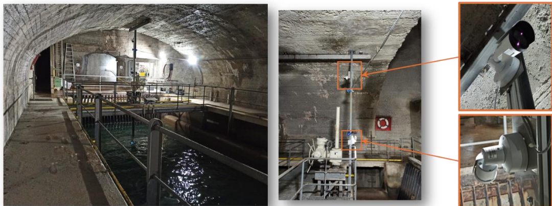
Figure 78 : Setup of the visual stroke measurement system installed on the pressure regulator piston of Unit 3 at KW Mörel .
