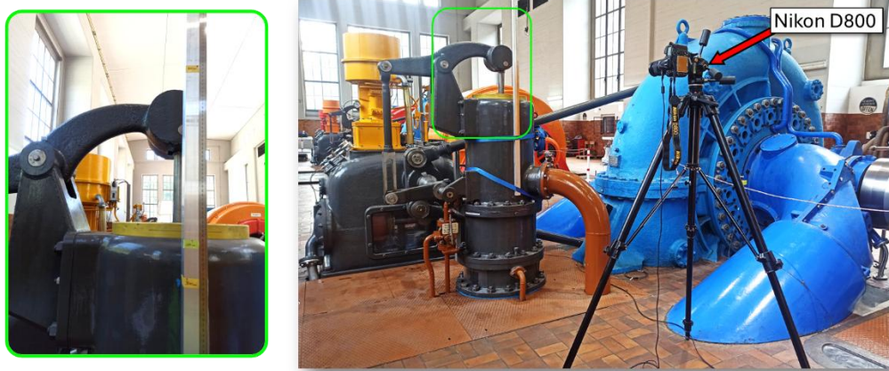
Figure 78 : Setup of the visual stroke measurement system installed on the pressure regulator piston of Unit 3 at KW Mörel .
