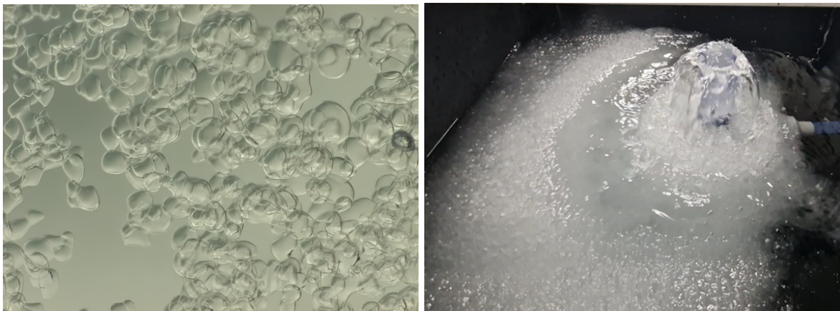
Figure 2: Left: ice slurry viewed through a microscope. (Source: Michael Froehlich). Right: ice slurry produced by the supercooling method. (Source: SPF - Institut für Solartechnik)
