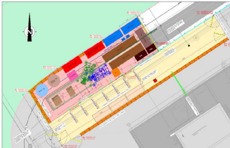
Figure 119 - Drilling site with inner (red) and outer (yellow) area
