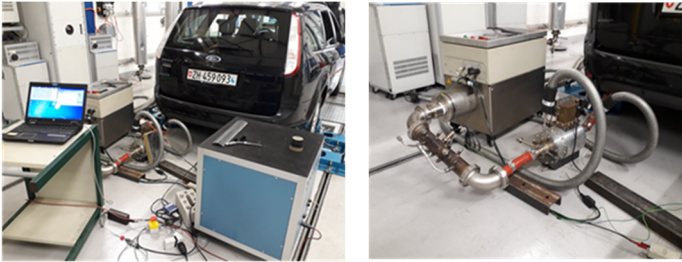
Figure (9) – Installment of the new catalytic converter at the end of a vehicle tailpipe on the chassi dynamometer.
