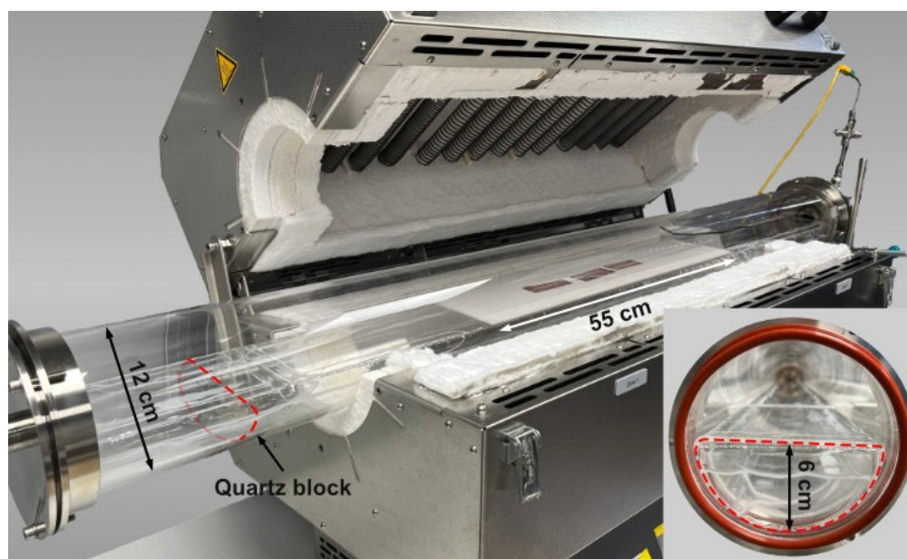
Figure 39. Picture of the modified ozone oxidation reactor hosting a quartz semi-cylindrical block (12 cm in diameter). The inset is the side view of the reactor with the quartz block
