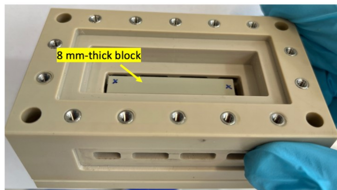
Figure 53. The block stuck in the membrane module to reduce the concentration polarization effect.
