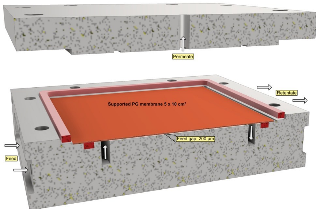
Figure 19. 3D design of the optimized membrane module with negligible concentration polarization effect.
