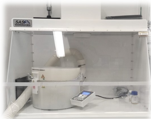
Figure 10. Large-area spin coater hosted inside a ventilated hood.
