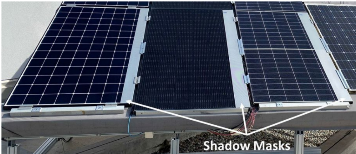
Figure 16: G/PERC/BS, G/IBC/BS and G/HJT/BS modules with shadow masks on the outdoor test stand.
