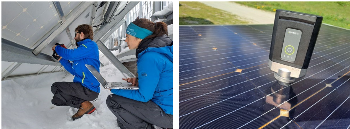
Figure 17: (left) FTIR-measurements of the backsheets of a PV installation at Dobratsch. (right) NIR measurement of a module.
