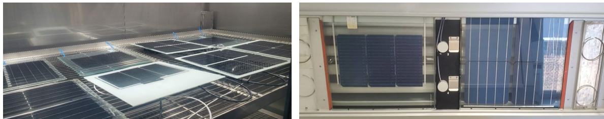
Figure 9: Mini-modules undergoing UV exposure. (left) Metal halide irradiation (300–2500 nm) at \approx 110^{\circ}\text{C} module temperature. (right) UVA irradiation (300–400 nm, intensified irradiance peak at 340 nm) at \approx 60^{\circ}\text{C} module temperature.
