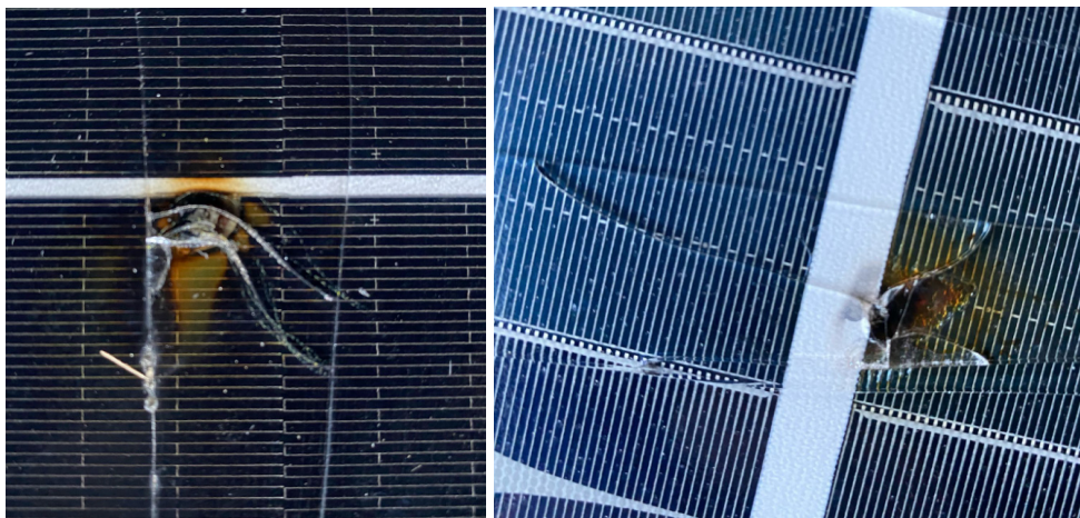
Figure 27: Close-up images on the thermally stressed areas and thermal fractures (wave-shape) of (left) front and (right) rear sides of the module in position #5.
