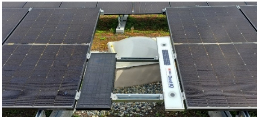
Figure 16: Soiling sensors installed: Intiyo sensor (left) and DustIQ Kipp&Zone sensor (right).
