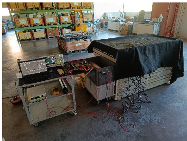
Figure 12: Dark I-V measurement set-up at SUPSI Mendrisio campus
