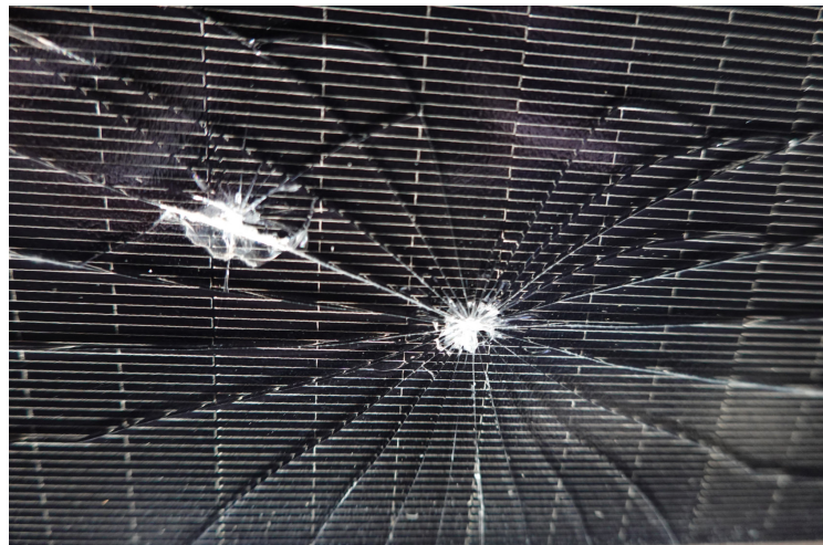
Figure 29: Front side of the impact on the module #14.
