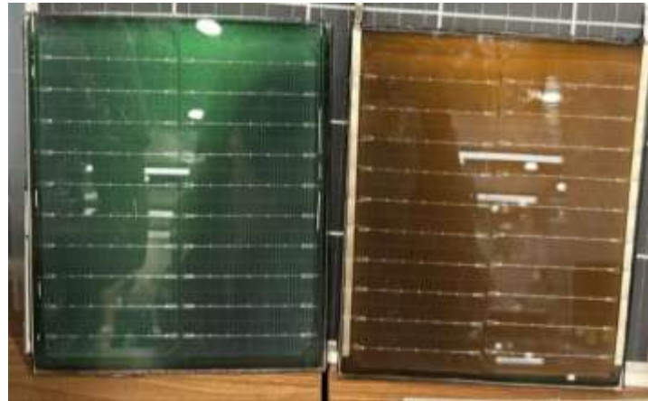
Fig. 43: Coloured PV mini modules produced at lab scale
