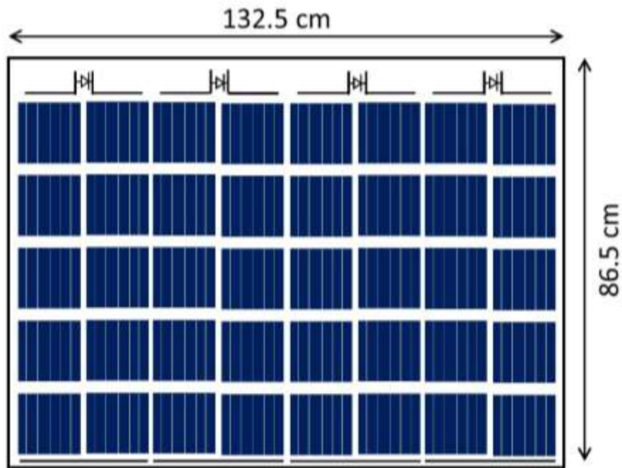
Fig. 34 Design of an upscaled module consisting of 40 series connected cells
