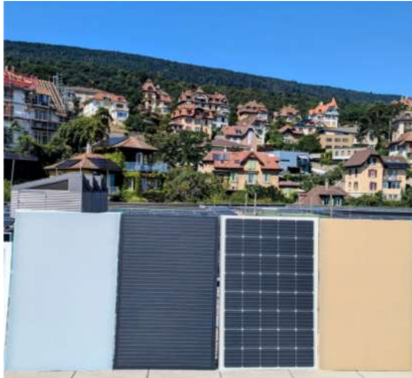
Fig. 35 Upscaled modules based on both PPGF8 and PPGF6 skins. The modules with beige and dark grey coloured foils are based on PPGF6 skins.
