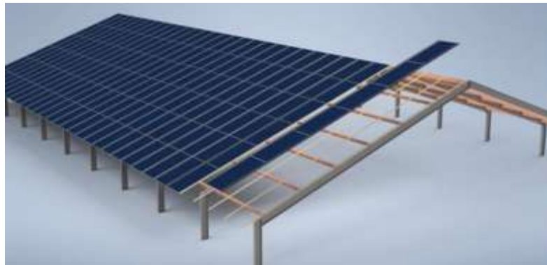
Fig. 1 Example of lightweight BIPV solution for agricultural, commercial, industrial roofs where standard PV solutions are not adapted due to weight limitations. Source: Solarge
