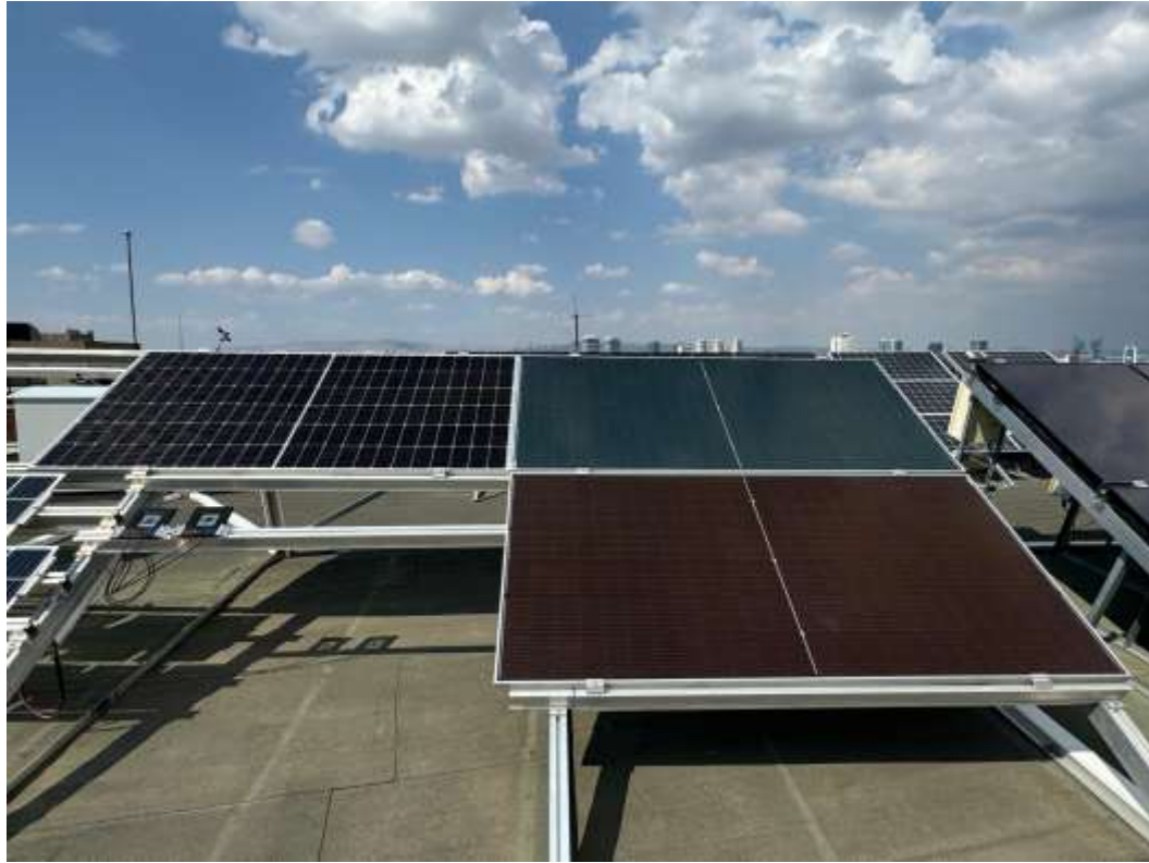
Fig. 47: Real image from the outdoor test center for the one-year I-V characterization monitoring service of the large-scale coloured modules produced.
