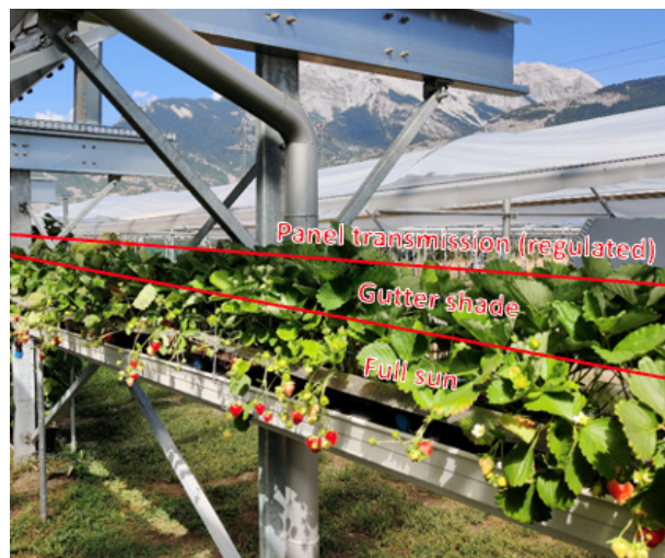
Figure 24: Photograph from the strawberry trial (02.08.2022), showing the light distribution on the plants, due to a sub-optimal positioning of the pots (rain gutter shading on the leaves, no shading on fruits).
