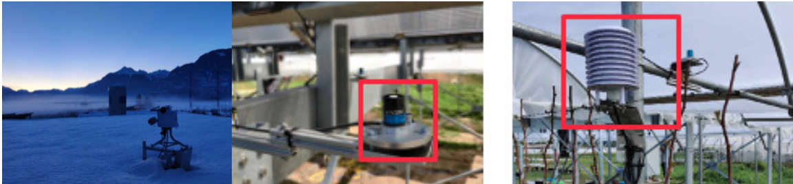
Figure 15: Climatic monitoring equipment deployed on site: Direct and diffuse irradiance sensor (left) ; Photosynthetically Active Radiation (PAR) sensor (middle) ; Temperature and relative humidity sensor (right)
