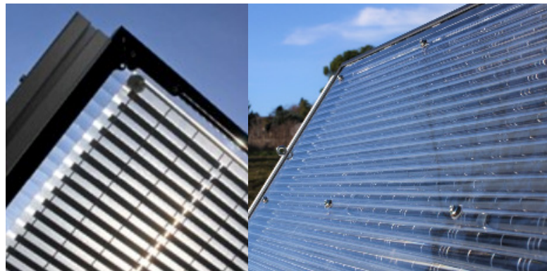
Figure 4: close-up pictures of the back side (with striped cSi cells) and front side (PMMA lens array) of the THEIA prototypes.
