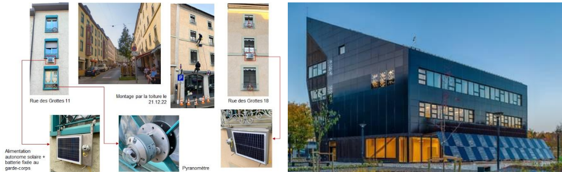
Monitoring of an urban canyon in Geneva with pyranometers (left), Zero Emission Building (ZEB) in NTNU
