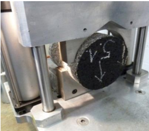
Figure 41: Testing of the layered composite according to Leutner method
