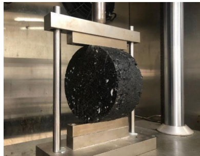
Figure 33: IDEAL-CT test setup and the principle of result expression from the load – displacement curve
