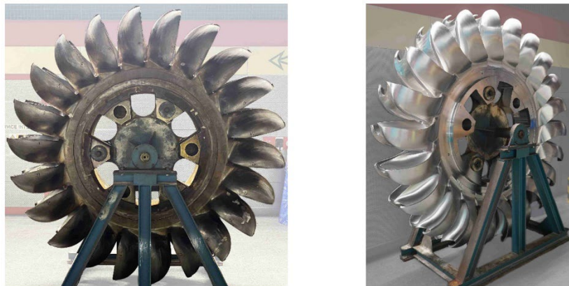
Figure 52: Geometries of the original runner (left) and new runner (right).
