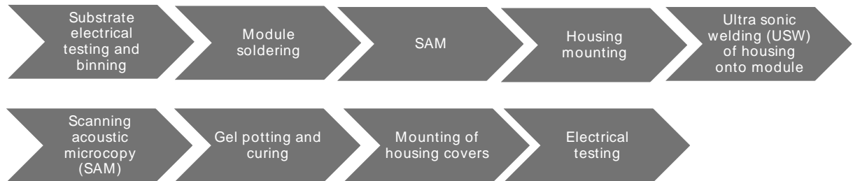
Figure: 34: Process flow of module assembly.
