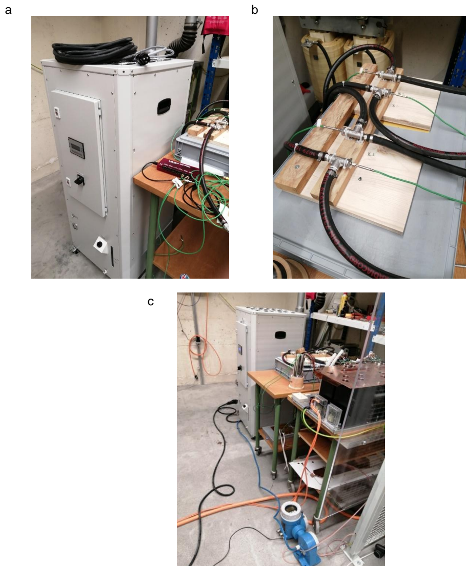
Figure: 62: (Top-left) Chiller unit. (Top-right) Thermocouples placed in the inlet and outlet of each coldplate. (Bottom) Power converter with cooling system.
