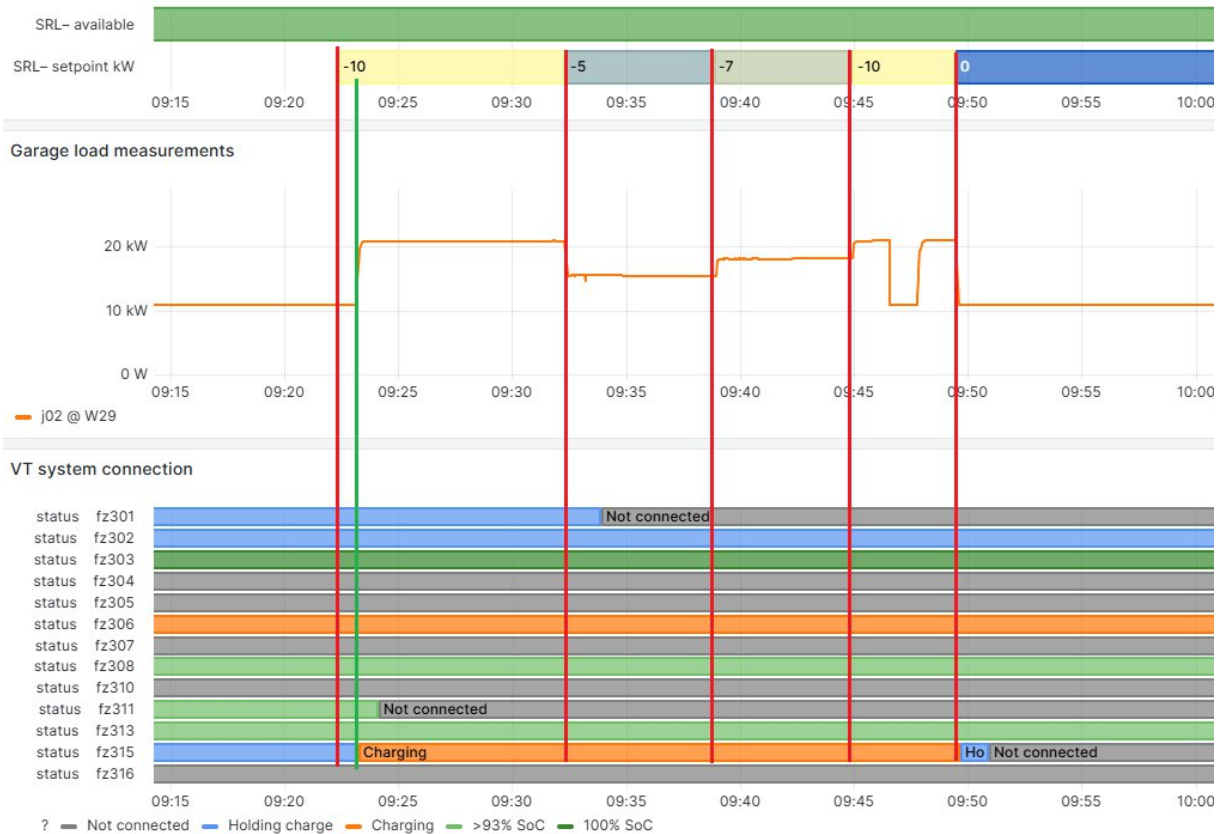
Figure 37. Ramps followed by available pool car for negative secondary control. Upper graph: Ancillary power request; middle graph: load measurement data from garage meter; lower graph: pool fleet vehicle status.
