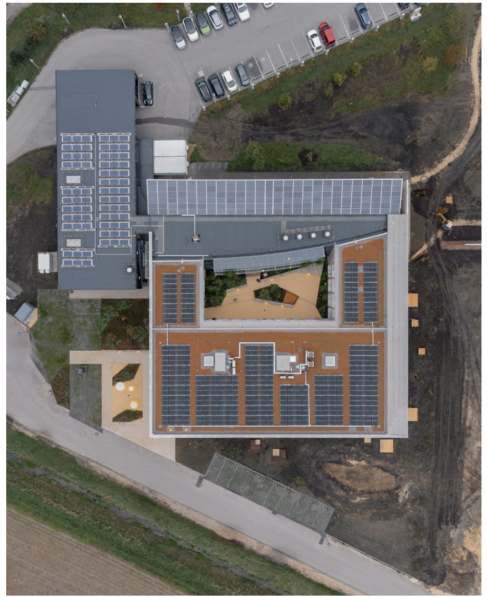
The Austrian company Windkraft Simonsfeld operates a number of wind power and solar power plants – and produces solar power itself at its headquarters in Ernstbrunn with a powerful PV system (70 kW). The GAMES project investigated how this can be used to power the company's own fleet of electric cars. Photo: Windkraft Simonsfeld
