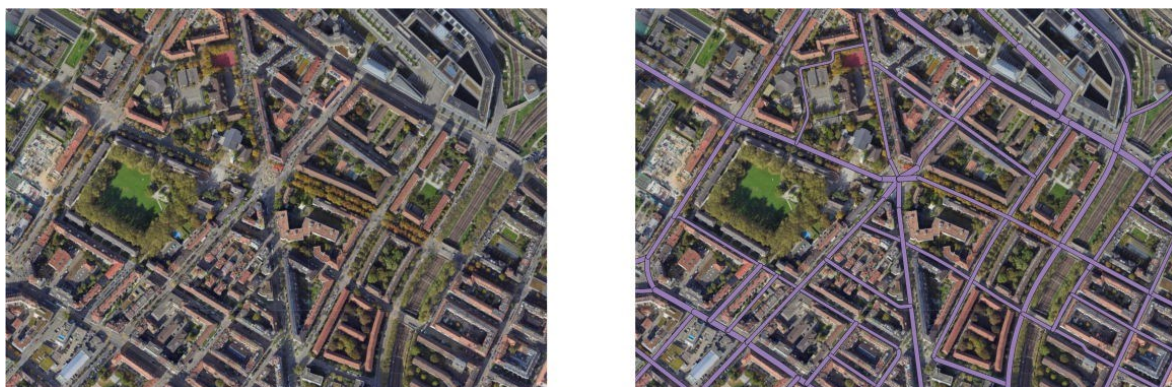
Figure 13: The aerial image (left) used as input to the machine learning model and the resulting road space estimation (right).
