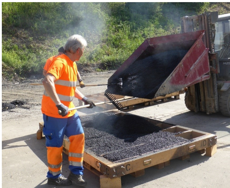
Figure 36: Collection of the asphalt mixtures AC 8 S and AC 11 S from an asphalt producing plant in Hinwil
