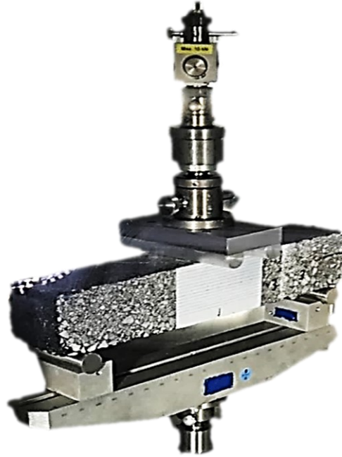
Figure 55: Test specimen mounted over 4PB bending beam loading assembly
