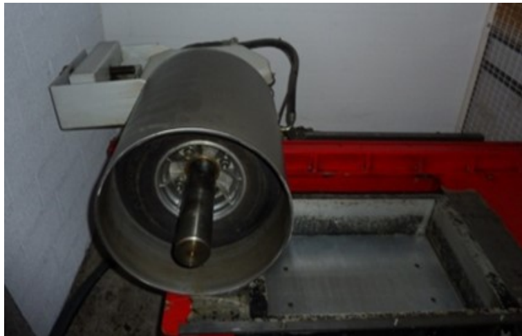
Figure 37: Modified compactor of the large device rutting tester
