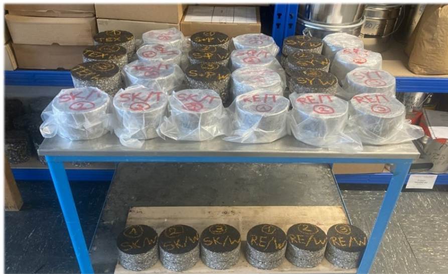
Figure 48: Laboratory Produced AST Specimens (Dry and Wet)
