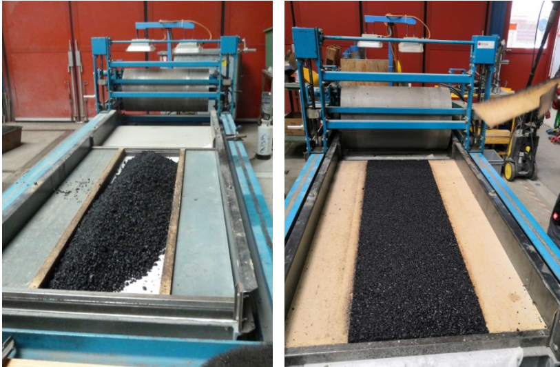
Figure 71: Roller compactor and specimen production for the MMLS3
