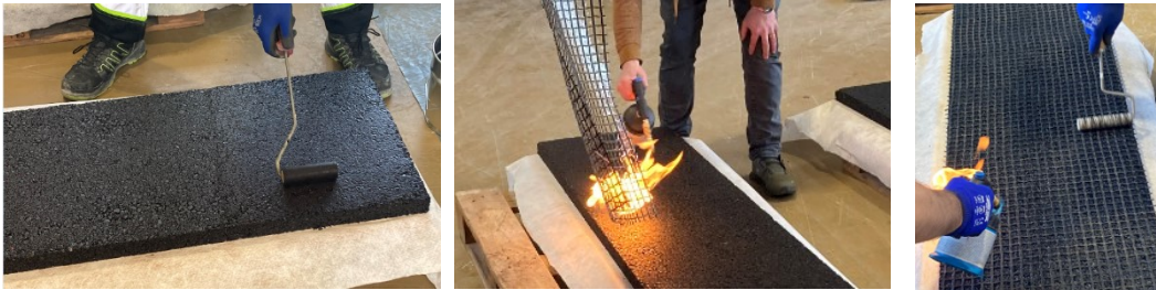
Figure 38: Application of System A
