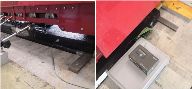
Figure 82: View of the thermocouples and data acquisition system
