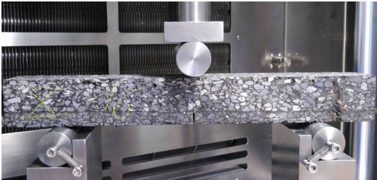
Figure 3: 3-point bending test
