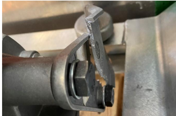
Figure 8-39 Rupture du second support moteur
