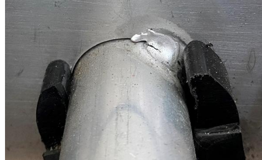
Figure 8-19 Soudure tub support lame 40 heures
