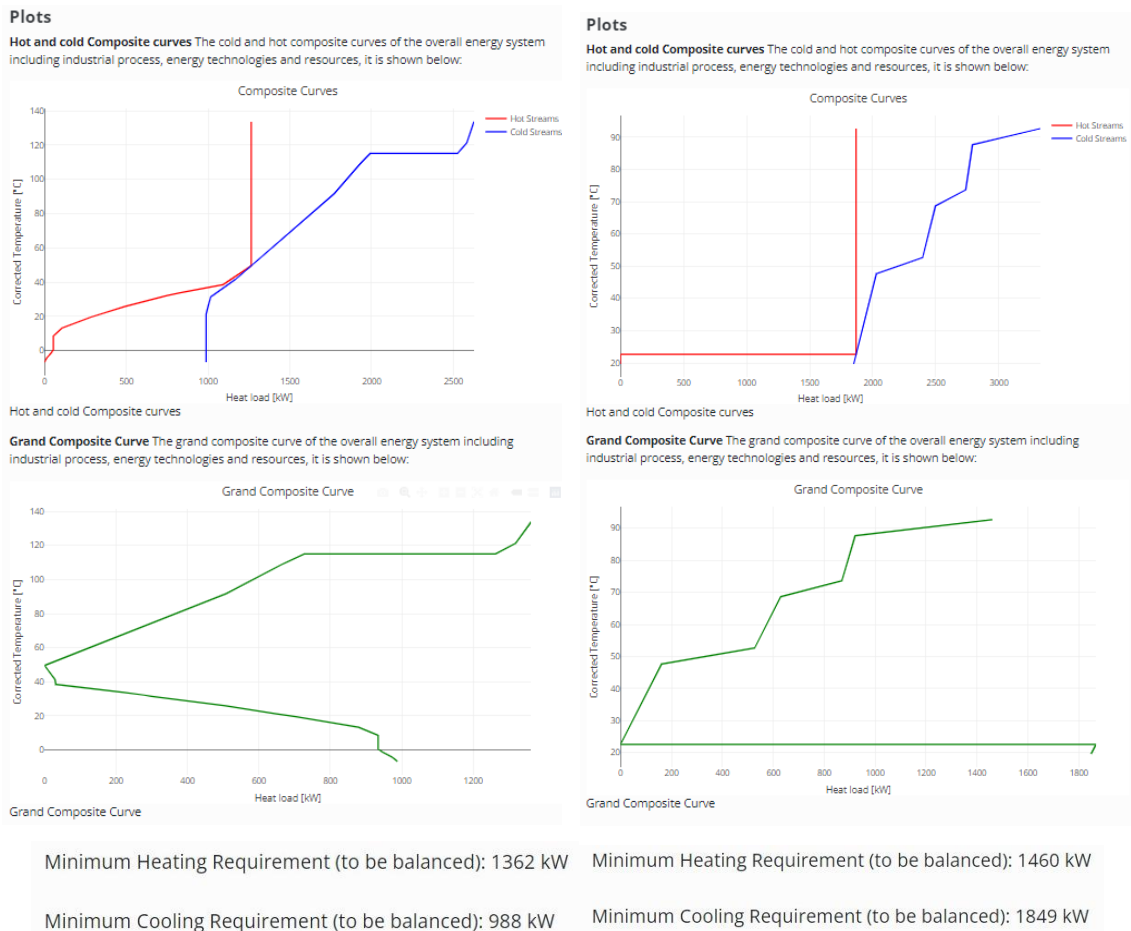
Figure 26: Composite (above) and gran composite curves (below) illustrate the estimation of the minimum energy requirement for Tixotherm (left) and CIP (right) processes.
