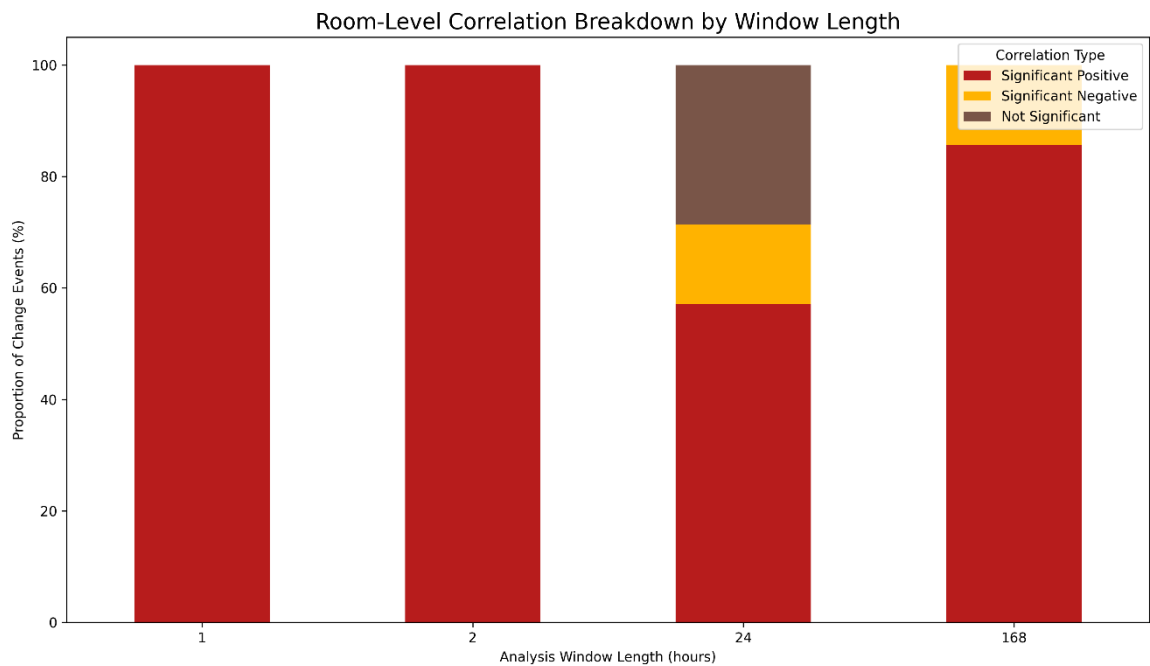
Figure 13: Direction and significance of the correlations between the changes in inlet temperatures and changes of the server room power consumption, grouped by the length of the analysis window.
