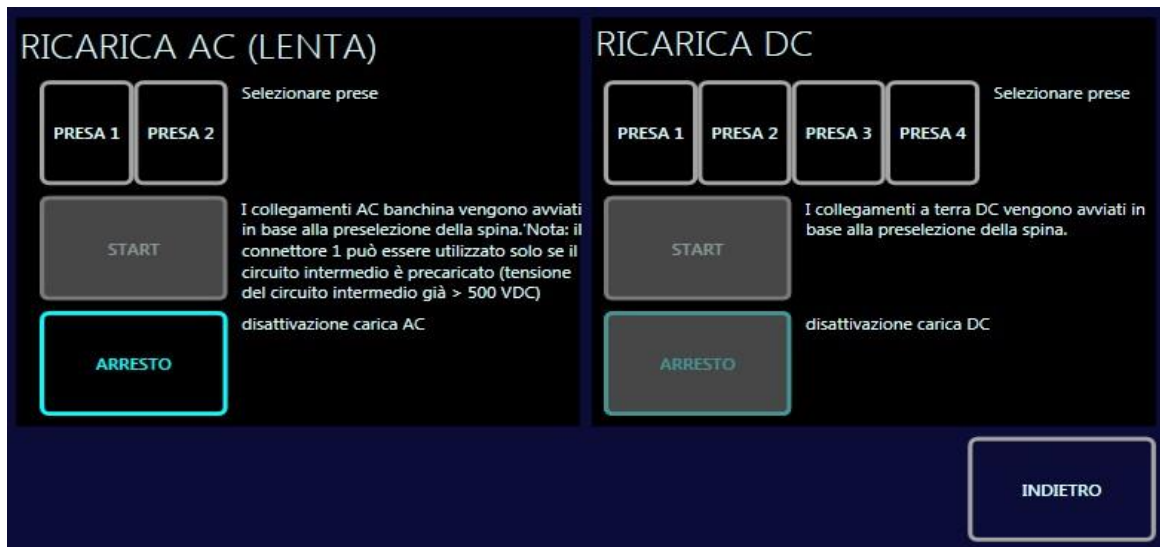
Figure 7 - HMI page on the control panel to choose the charge method
