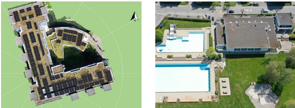
Figure 2. Visualization and aerial footage of a retirement home and the indoor swimming pool in Wittenbach (Isler et al., 2024). Several variants for each building were designed and analyzed with power ratings between 99 and 111 kWp on the retirement home and between 147 and 198 kWp on the indoor swimming pool.
