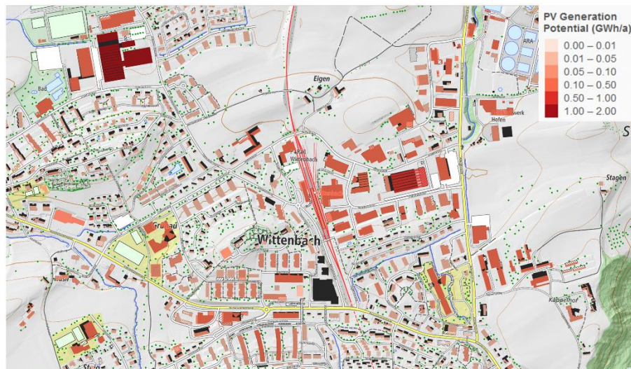
Figure 1. Illustration of results of geolocated analysis of PV potential on roofs of buildings in Wittenbach. A building consists of an arbitrary number of individual roof areas, which were grouped together for this analysis. Reduction factors were previously applied to the individual roof areas as described in section 2.1.
