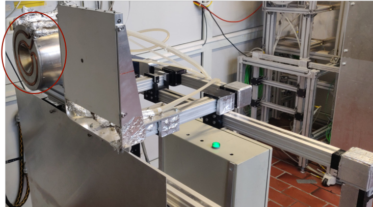
Figure 9: An image of the calorimeter setup is shown. The red oval highlights the front of the calorimeter, which is facing the HFSS.
