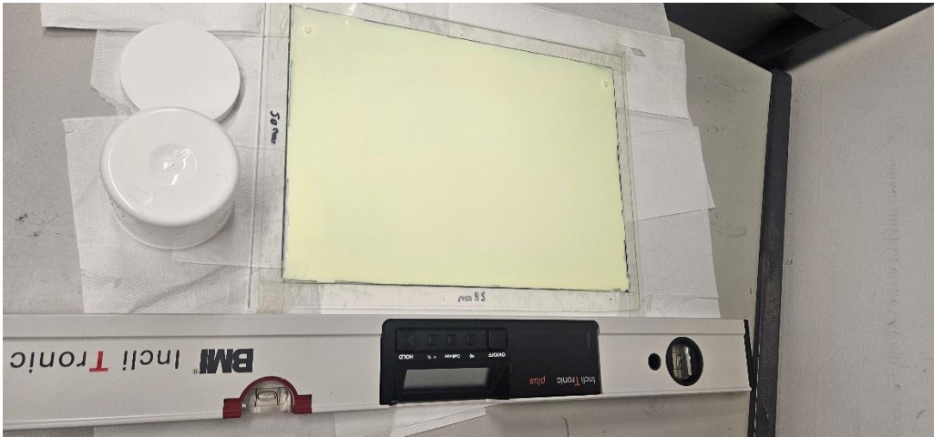
Figure 3 LSC Plextol 455 with 0.2wt% BY40 on a glass plate.
