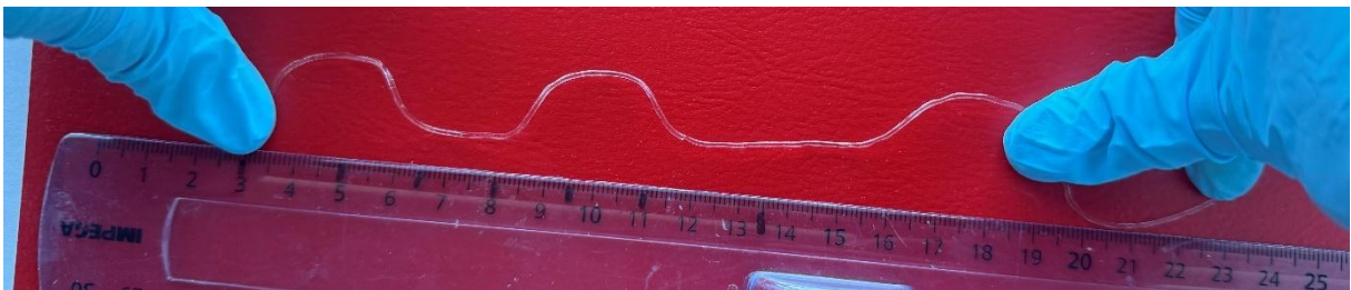
Figure 21 APCN fiber made of 30wt% HEA and 70wt% DDDMA.
