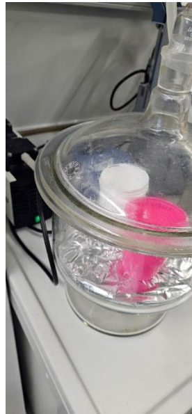
Figure 1 a) Sylgard 184 and Tubcosil HAB5-1 were put in a desiccator to remove the air bubbles before coated on PES.
