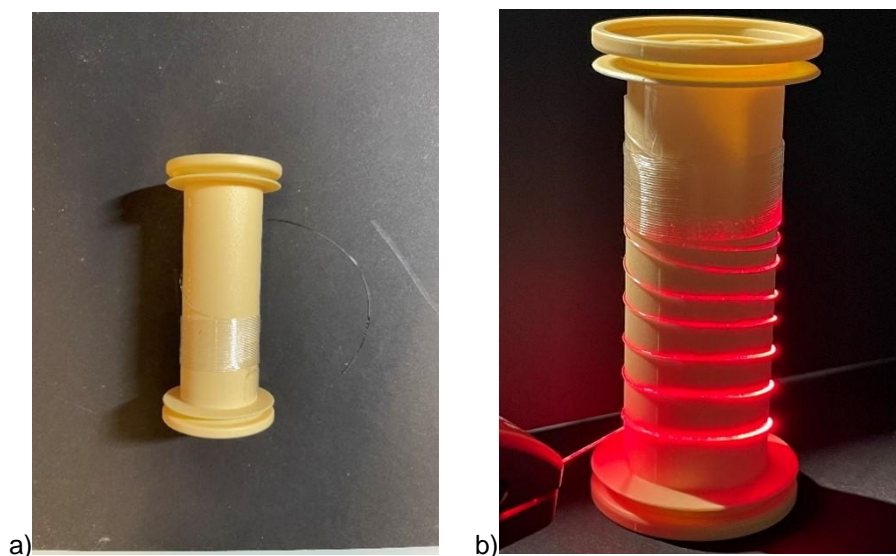
Figure 18 a) Microfluidic spun acrylate fibers rolled up on a spool. b) Light guided through an acrylate fiber obtained from microfluidic spinning.
