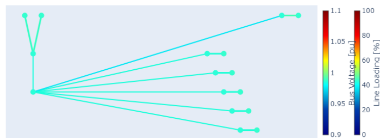
Abbildung 21: The overview of power flow results of the synthetic grid.
