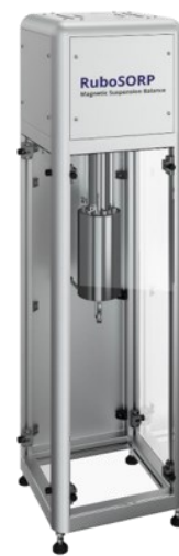
Figure 5. High-pressure sorption analysis system Rubosorp 700 with the basic layout (PFD) on the left, the main control unit containing the valve blocks (middle), and the actual measurement cell (right).
