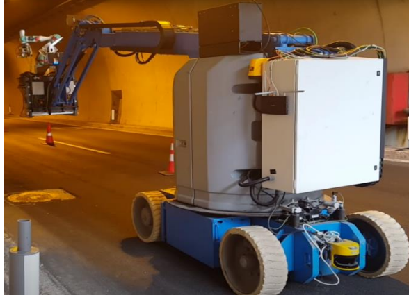
Abb. 7 ROBO-SPECT: Robotic System for tunnel structural inspection & evaluation [56]
