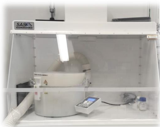
Figure 5. Large-area spin coater hosted inside a ventilated hood.
