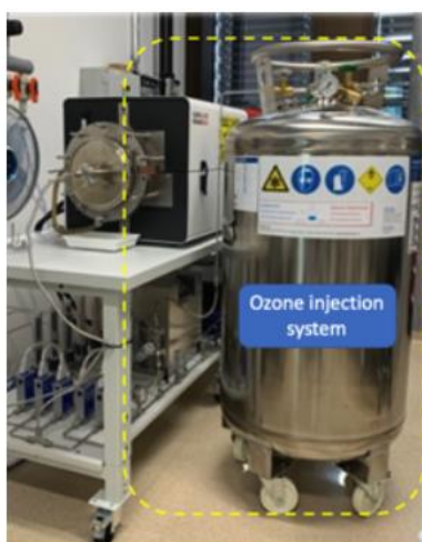
Figure 20. Ozone reservoir for a quick injection of ozone into the CVD furnace.
