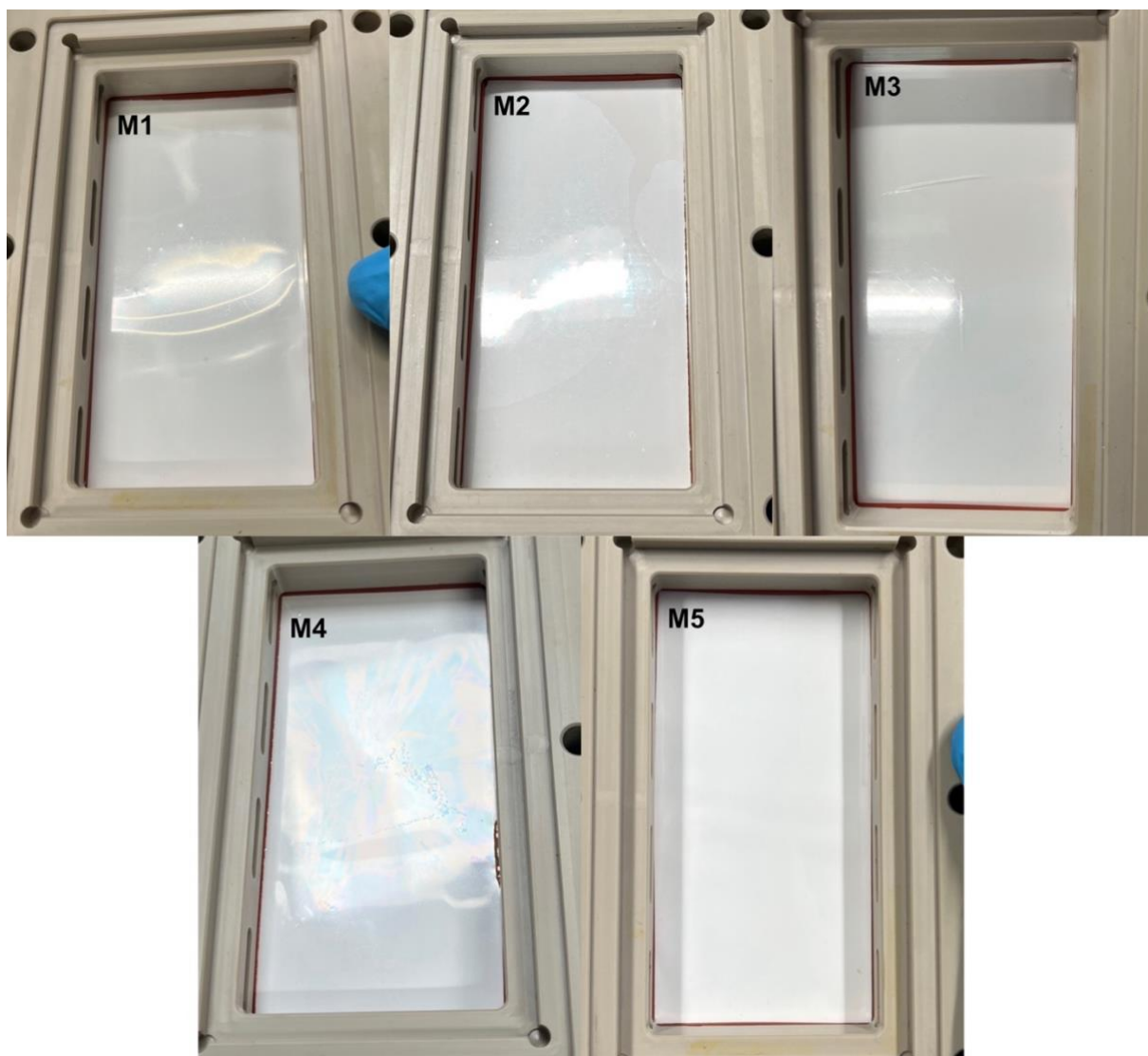
Figure 39. Pictures of five 50 cm 2 porous graphene membranes.
