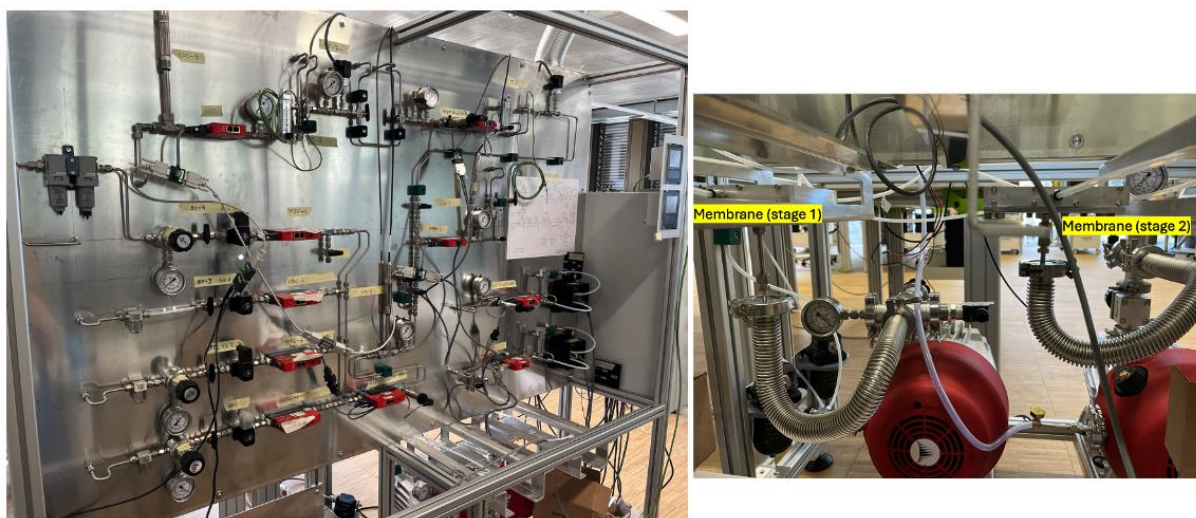
Figure 10. The two-staged membrane skid (left). Right: The two membrane modules are highlighted on the right.
