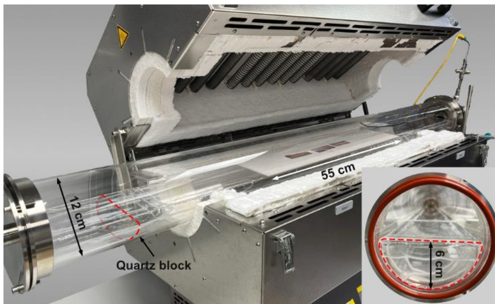
Figure 35. Picture of the modified ozone oxidation reactor hosting a quartz semi-cylindrical block (12 cm in diameter). The inset is the side view of the reactor with the quartz block
