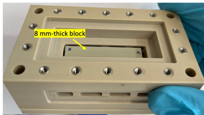
Figure 48. The block stuck in the membrane module to reduce the concentration polarization effect.
