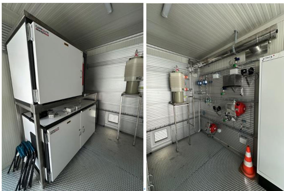
Figure 60. Membrane skid for testing graphene membranes for the separation of flue gas from combined heat and power (CHP), installed in Aigle under the premises of GAZNAT.
