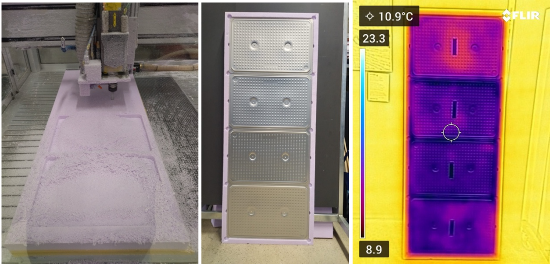
Figure 28. CNC processing of XPS (Left); Functional test (Right)
