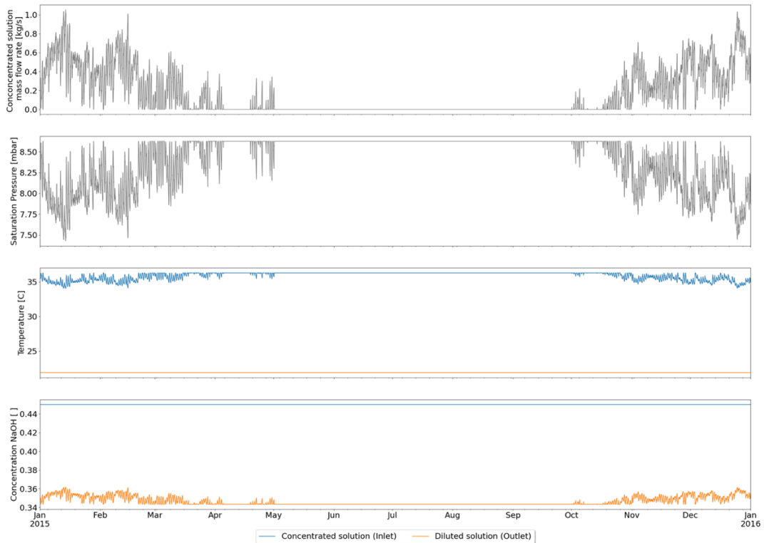
Figure 64. CS1 – Closed-sorption reactor operation
