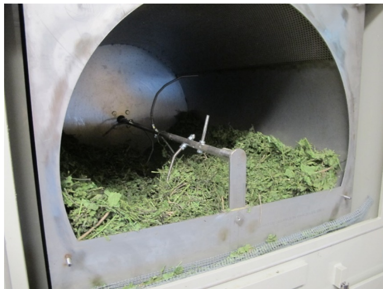
Figure 25: Project “Sonitro” drying chamber for tea leaves with agitator.
