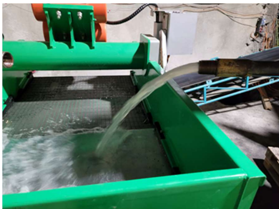
Figure 2. Open ended flow test of the surface system over the shaker
