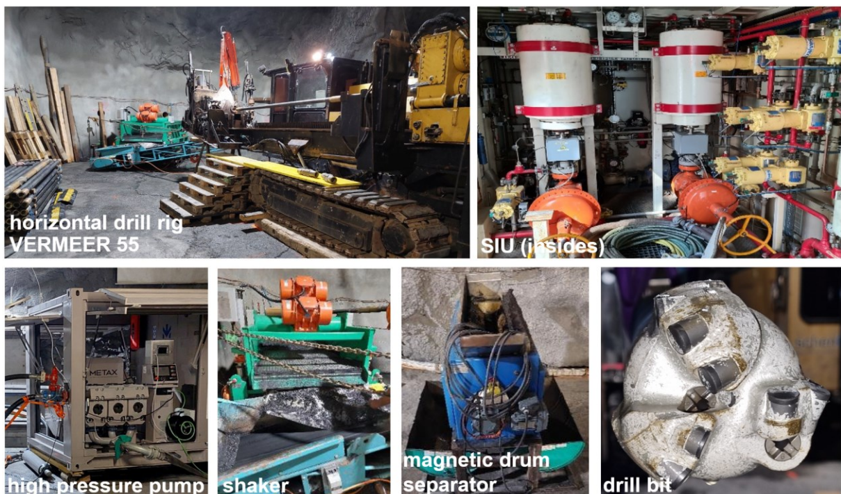
Figure 3: Overview of key operational equipment deployed during the trial at VSH test site.
