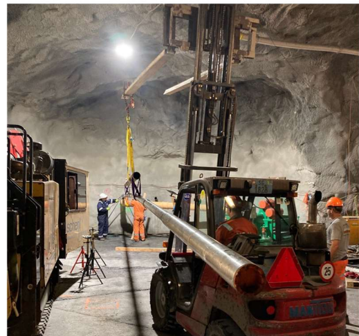
Figure 1. Overview of the drill site (left) and making-up and running-in-hole the 'empty' drilling assembly without electronics (the internal 'jewelry') (right).
