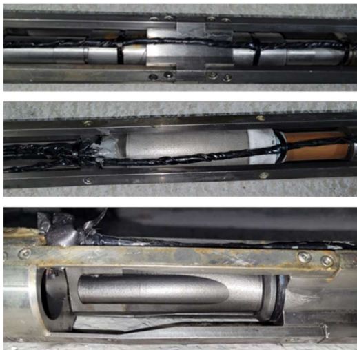
Figure 17. Inspection of the steering sub internals: Centralizers (top) and sensors (middle) undamaged. Cable at rotor damaged (bottom).
