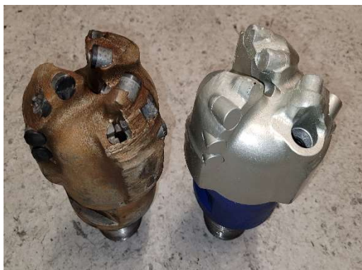
Likely scenario is that the bit ran into a layer of quartzite at a very shallow angle. The bit is rated up to 7 daN weight, but when only a few cutters are exposed to that force they will break down. The cutters at medium radius are most exposed to the pushing force and remove more rock than the inner cutters. With a harder, abrasive layer coming from the side only one or two cutters were likely to be exposed to the full pushing force which may damage them.
