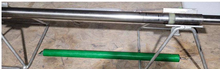
Figure 19. Replacing the battery (green) for the steering sub in its housing.
