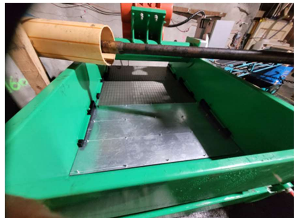
Figure 5. Modified shaker screen for suppressing leakage of steel shot underneath the scatter plate
