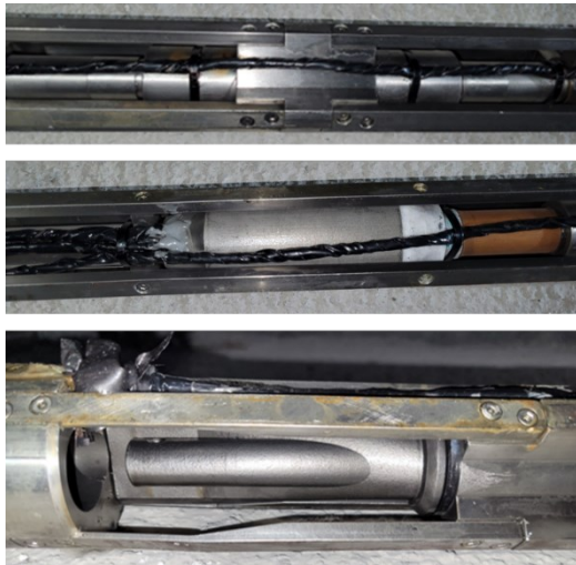
Figure 4: Internals of the steering sub showing centralizers (top), sensors pack (middle), and the rotor (bottom)
