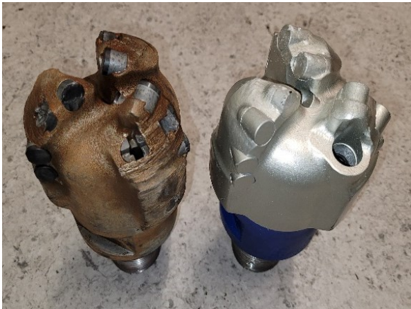
Figure 10: Used bit (left) vs. an unused bit (right). The used bit had several cutters at medium radius heavily damaged.
