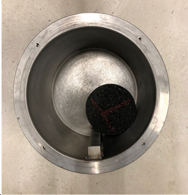
Fig. 26 Test setup for the MDI test. With every revolution, the sample has to roll over the obstacle
