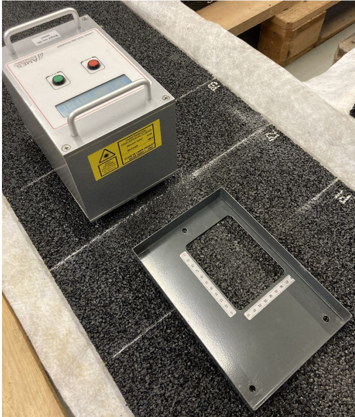
Fig. 30 Evaluation of asphalt slab with Ames Engineering 9400HD 3D laser scanner
