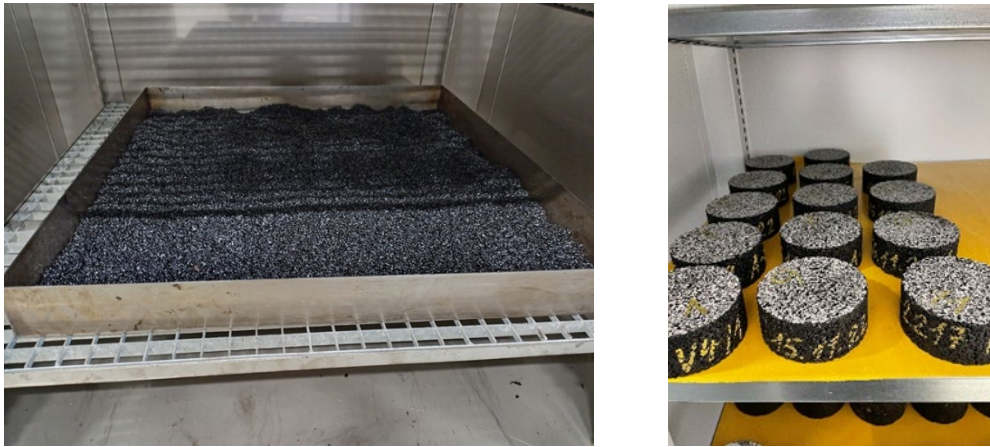
Fig. 21 Short term oven aging on mixture left and compacted and cut samples, right
