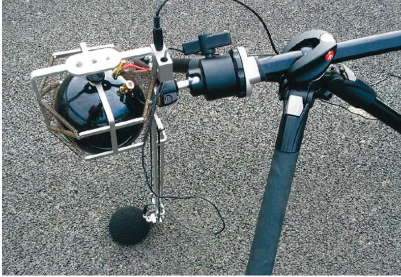
Fig. 31 Sound absorption measurement device “PU-Probe” on a low noise road surface. The loudspeaker is shown on the upper left corner, while the PU-Sensor is situated on the road surface
