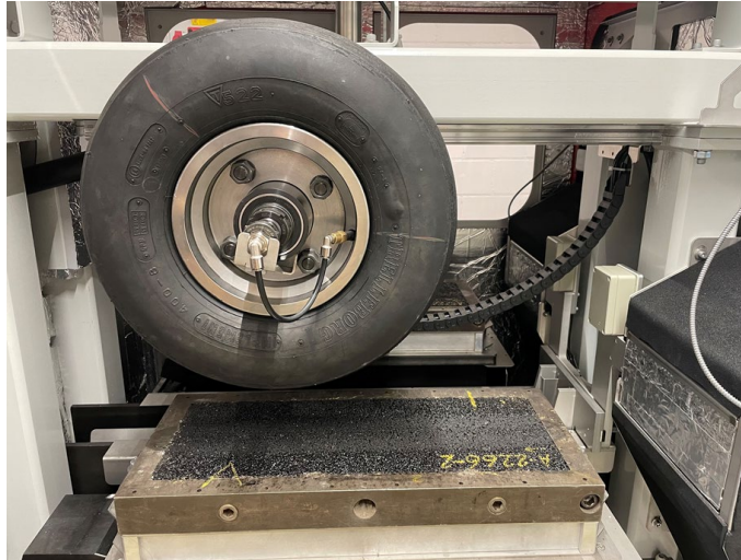
Fig. 22 French rutting test set up
