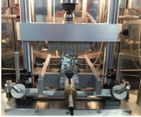
Fig. 24 Experimental set up for the stiffness modulus and fatigue tests
