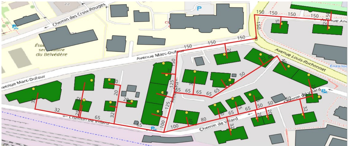
Figure 91 : Nominal diameter integrated into each of the District Heating Network pipes in the first scenario
