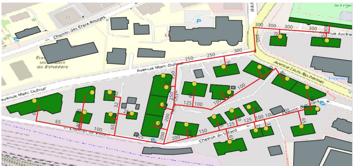
Figure 100 : Nominal diameter integrated into each of the DHN pipes in the third scenario
