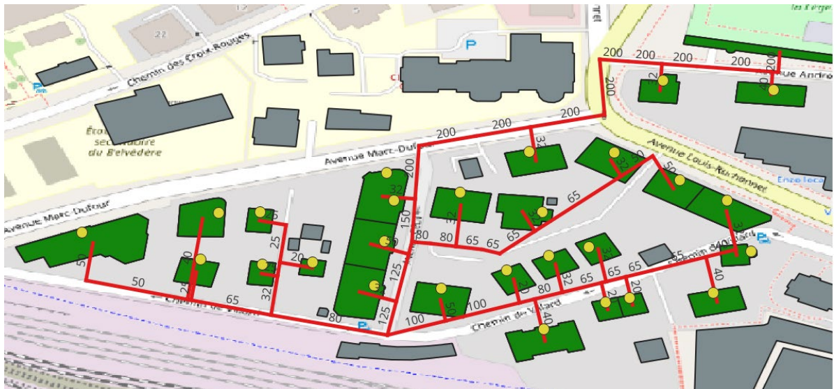
Figure 97 : Nominal diameter integrated into each of the District Heating Network pipes in the second scenario
