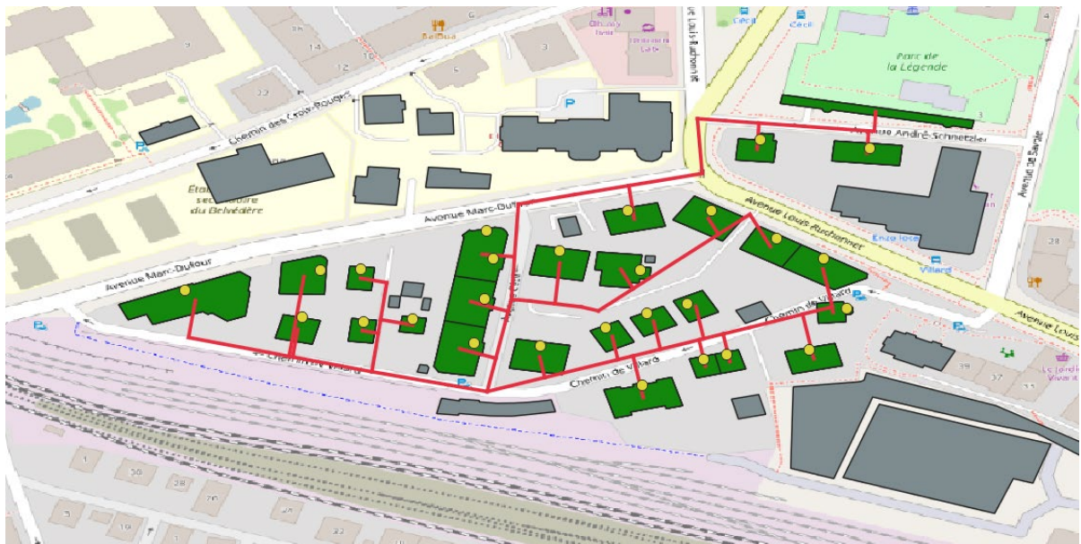
Figure 90 : Visual representation of the designed District Heating Network (DHN) with connections
