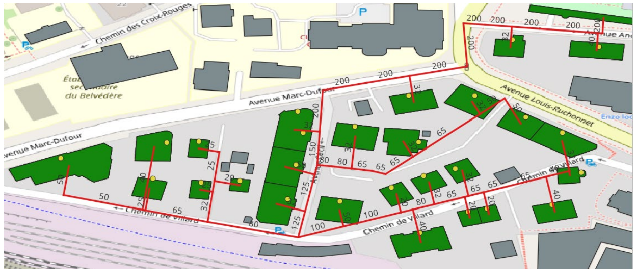
Figure 102 : Nominal diameter integrated into each of the DHN pipes in the fourth scenario
