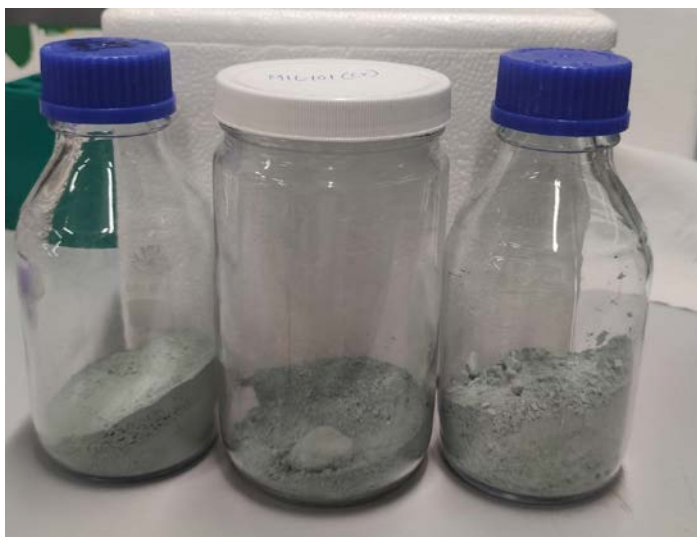
Figure 15: Approximately 250 g of Cr-MOF, made in 13 batches.
