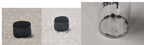
Figure 37. (Left) Pellet of support containing TEPA-BDE before and after friability test and (right) pressed mesoporous powder.
