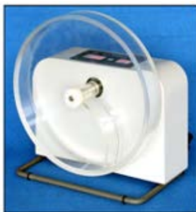
Figure 9. Picture of the attrition instrument that will be used in the future to assess the robustness of the structured adsorbents.
