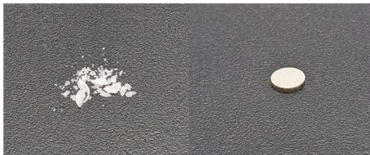
Figure 33. Pellet of bare KIT-6 (left) and PEI-grafted KIT-6 (right).
