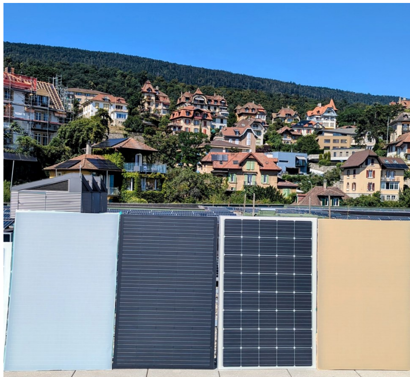
Fig. 28 Upscaled modules based on both PPGF8 and PPGF6 skins. The modules with beige and dark grey coloured foils are based on PPGF6 skins.
