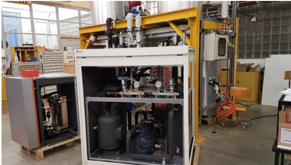
Figure 35 Transcritical HP Enex GeoHeat 18 under test in the HEIG-VD lab.
