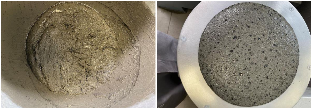
Figure 12: bleeding of Carbonova CNF in freshly mixed mortar (left) and slump flow cake (right).
