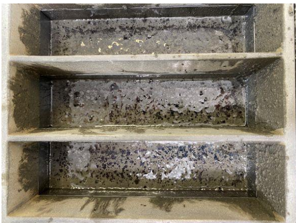
Figure 13: Bleeding of Carbonova CNF in prism molds right after casting.
