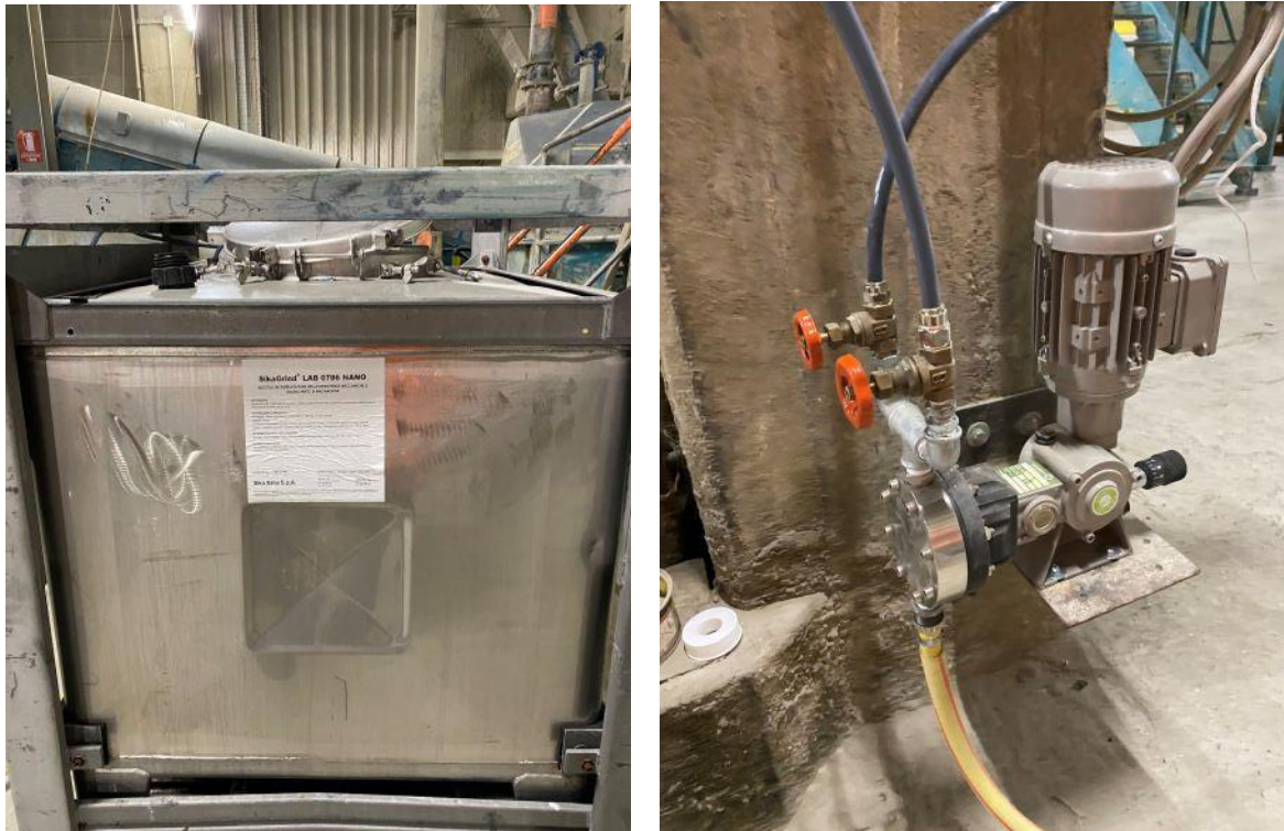
Figure 9: IBC (left) and pumping/recirculating system (right) of the graphene slurry during the trial.
