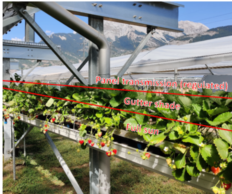
Figure 23: Photograph from the strawberry trial (02.08.2022), showing the light distribution on the plants, due to a sub-optimal positioning of the pots.
