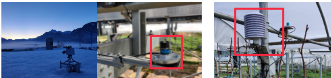
Figure 16: Climatic monitoring equipment deployed on site: Direct and diffuse irradiance sensor (left) ; Photosynthetically Active Radiation (PAR) sensor (middle) ; Temperature and relative humidity sensor (right)
