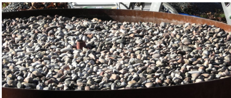
FIGURE 2: TOP SURFACE OF THE PACKED BED AFTER THE VIBRATION PROCESS.
